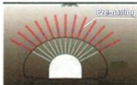
(a) Soil nailing with grouting
