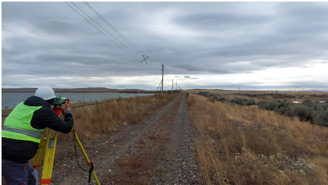
Figure 5 – Leveling is a key step in validating digital models and controlling vertical displacements.
