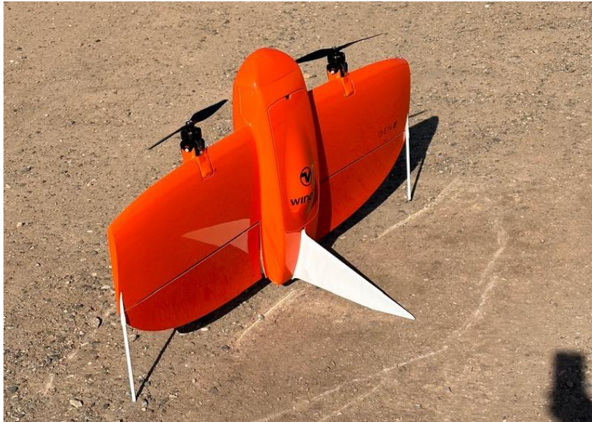
Figure 6 – Vertically launching UAV used for detailed aerial surveys.
