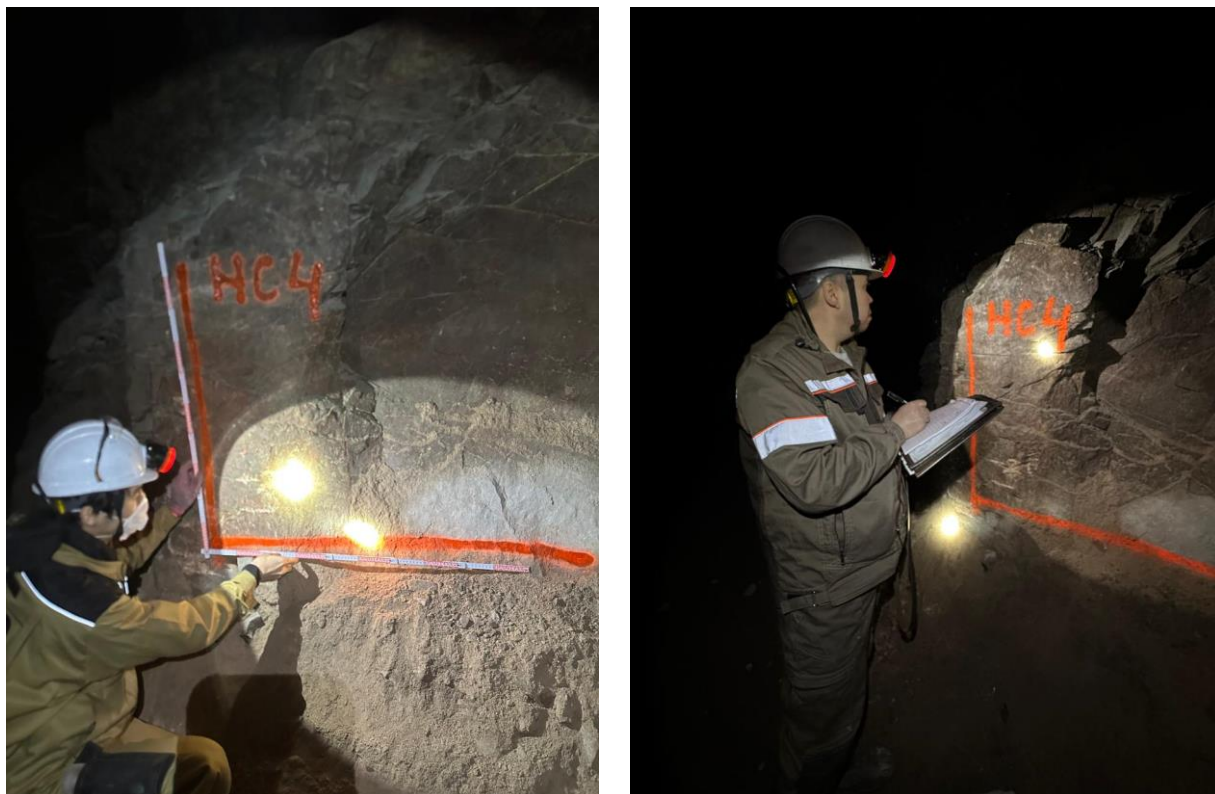
Figure 1 – Underground investigations for determining the structural characteristics of rock formations
