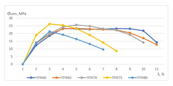
**Figure 2** – Deformation-strength dependences during uniaxial compression of PPK samples filled with quartz filler in the range of 60...80 wt.%
