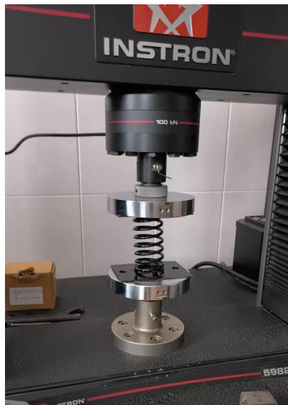
Figure 10 – Testing of elevator bumpers and vibration isolators
