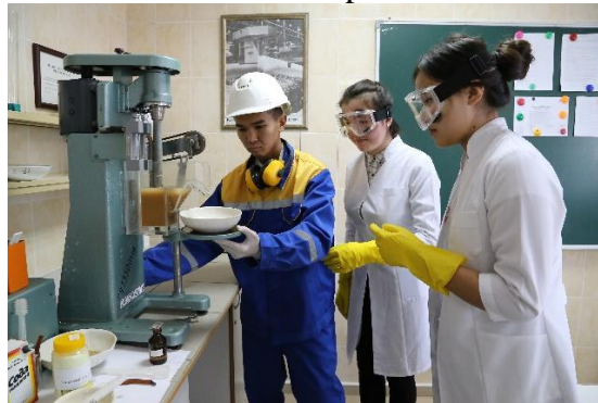
Students of the OP "Mineral enrichment" carry out foam flotation on a flotation machine and receive copper concentrate (2020). In the photo: Amangeldinov A.A., Shakenova A., Bektasova N.
