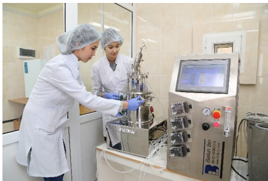
The process of adding a nutrient medium to a bioreactor for culturing microorganisms (2020).
